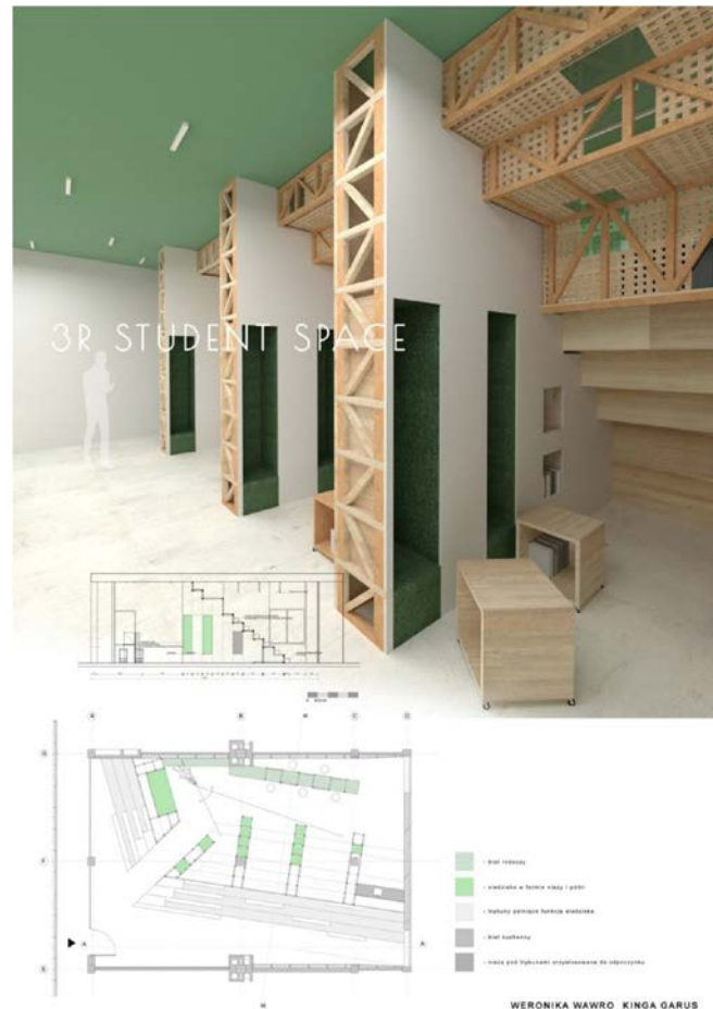
Figure 2: Resources efficiency design strategy accomplished through the dematerialisation of interior components and multifunctionality of interior structures (authors: W. Wawro and K. Garus; supervisor: M. Celadyn) (source: Archive of the Faculty of Interior Design, Jan Matejko Academy of Fine Arts in Kraków).
